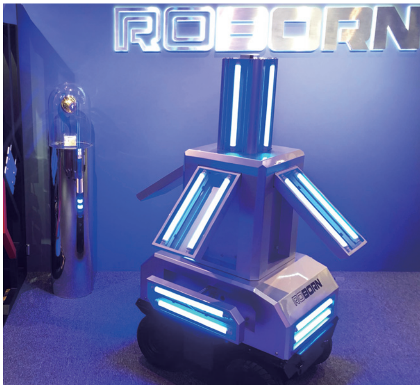
最新研發的消毒機械人，會自動行走並以 UV 燈消毒四周。 A latest development, this robot can move about automatically and disinfect its surrounding area with UV light.
